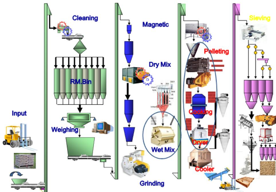
Figure 3: Process diagramme of shrimp feed production
