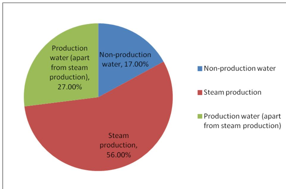
Figure 5: Water use in the representative factory
