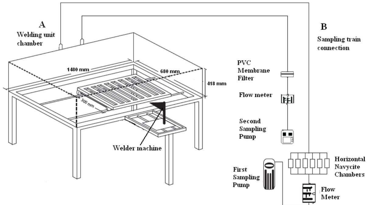
**Figure 1:** Automated welding unit chamber
