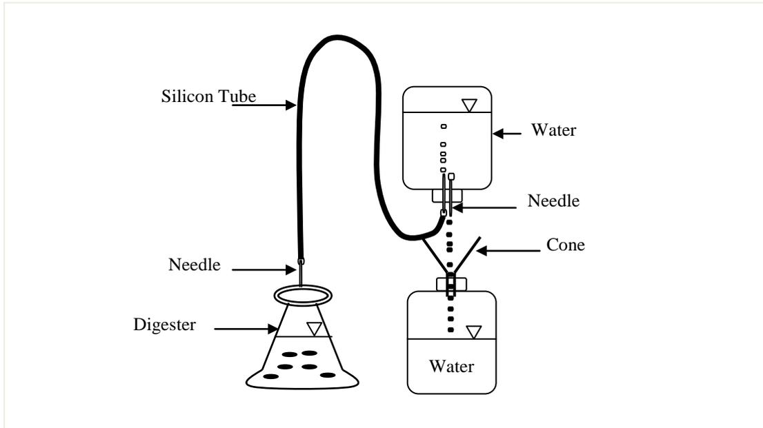
**FIGURE 1:** Schematic diagram of the digester.
