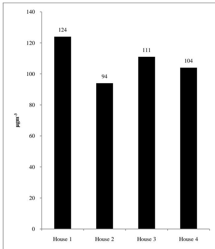
FIG. 4- Mass concentration of indoor PM<sub>10</sub> in selected terrace houses
