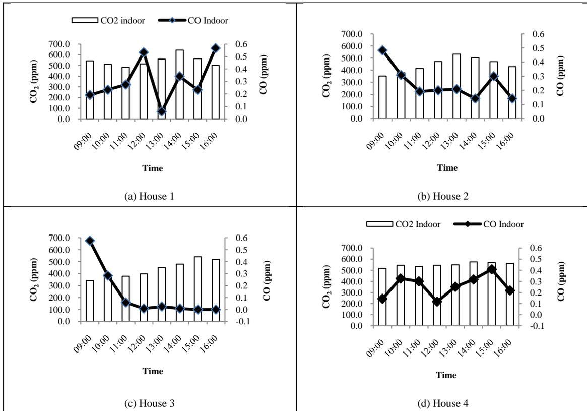
FIG. 3- Indoor carbon dioxide (CO<sub>2</sub>) and carbon monoxide (CO) profile in selected terrace houses
