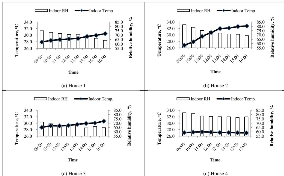
**FIG. 2-** Indoor temperature and relative humidity (RH) profile in selected terrace houses
