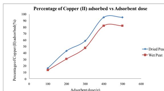
**FIG. 1-** The effect of peat quantity on absorption of Copper
