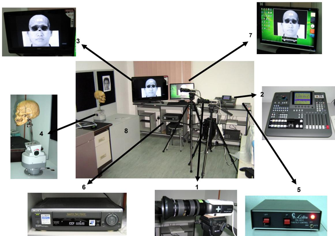
**FIG. 1-** Components of the Computer Aided Video Superimposition Device (CAVSID) fabricated in Universiti Sains Malaysia, the first of its kind in Malaysia.
