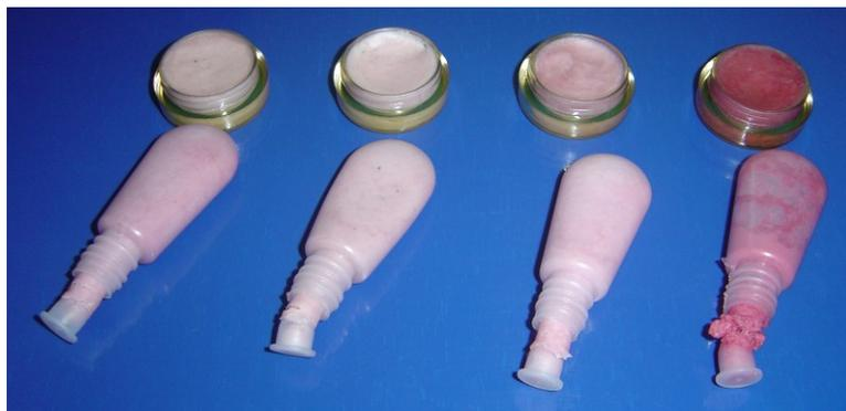
FIG. 3- The texture of the irradiated lip balms became harder and cannot be pressed out from the tubes.
